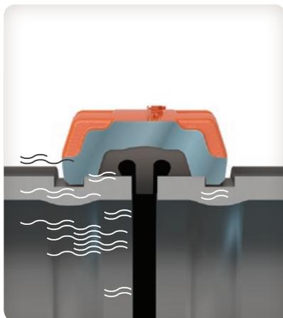
**Noise and vibration attenuation** – by isolating the transference of vibration at each joint.
