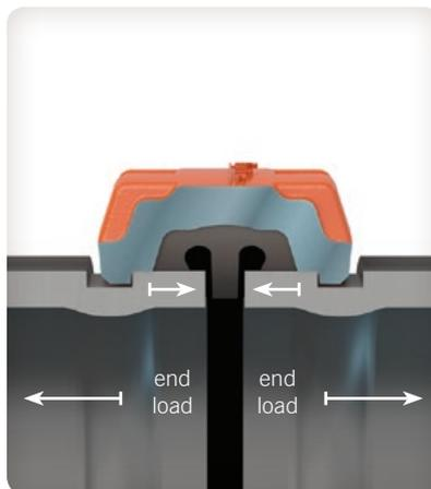
**Self restrained pipe joints** – couplings engage the pipe grooves to hold the pipes against full pressure thrust loads without the need of supplemental restraints.
