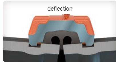
**Flexibility** – with the inherent axial movement and deflection properties of flexible couplings in a groove system. May be used to accommodate pipeline thermal expansion and contraction, misalignment and settlement, and seismic stresses.
